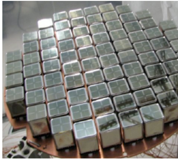
242 (Hamamatsu R8520) 1"x1" low radioactivity PMTs
