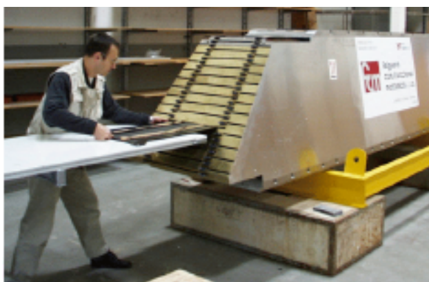
Insertion of tiles into wedge
