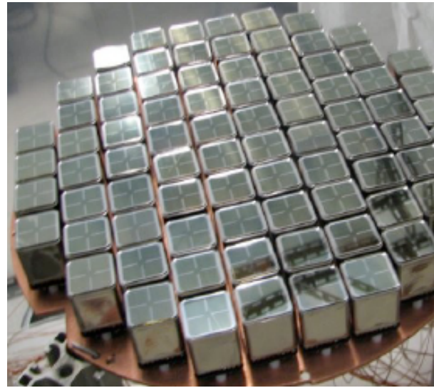
242 (Hamamatsu R8520) 1"x1" low radioactivity PMTs
