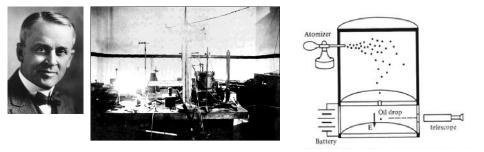
By measuring the free fall of tiny olive droplets in air, Millikan estimated the electron charge and, taking the Thomson result on e/m, evaluated electron mass:
