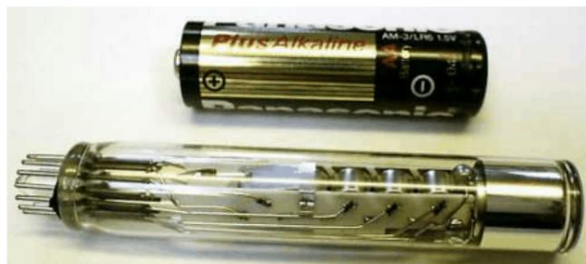
Single photon, if it produces the first electron (photoelectric effect) results in macroscopic charge.
