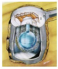
Large tank with 7000 t of water  $(H_20)$ Sphere with 1000 t of **heavy water**  $(D_20)$
