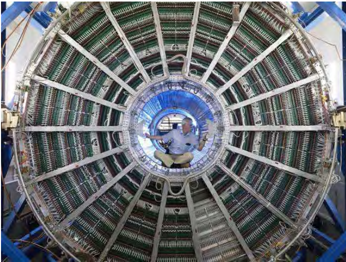
TPC endcap, readout sectors are visible
