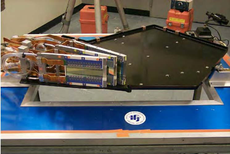
Support structure for the multi-layer Si spectrometer
