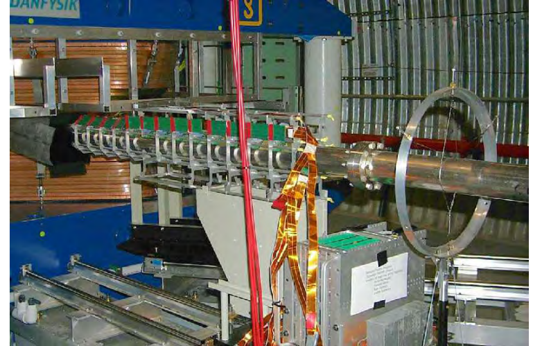
Support structure for the octagonal multiplicity detector
