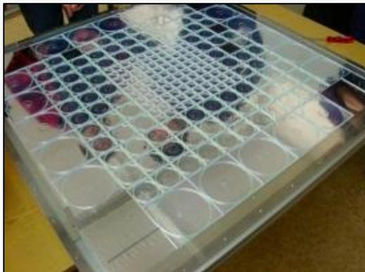
**AHCAL** tiles and SiPMs for technological prototype
