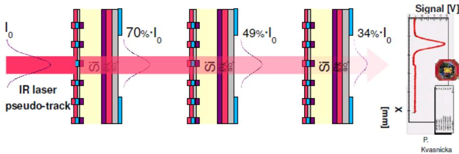
*Improved InfraRed transparent microstrips detectors for tracker alignment*
