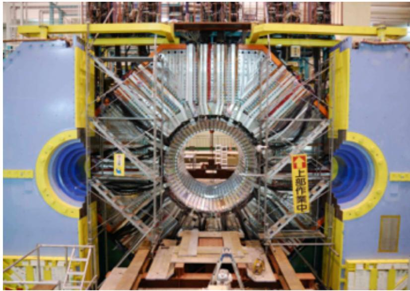
Belle detector was positioned in the assembly hall next to the collision hall, for the major upgrade (8 meters each, weight: 1400 ton)
