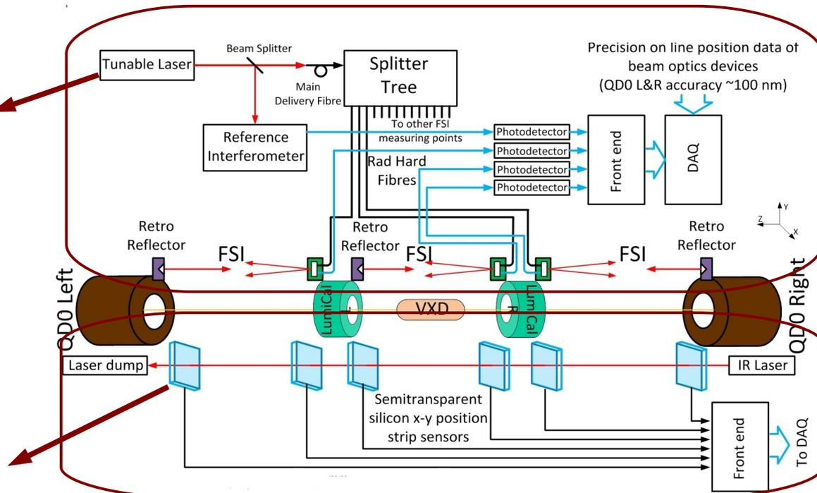
FSI – using tunable lasers will measure the absolute distance between LumiCal calorimeters by measurement of interferometer optical path differences (counting the fringes)
