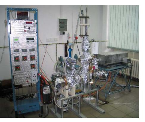
to achieve good superconducting film properties the partial pressures of water, nitrogen, oxygen,  $CO_2$  hydro-carbides etc., must remain well below  $10^{-9}$  hPa
