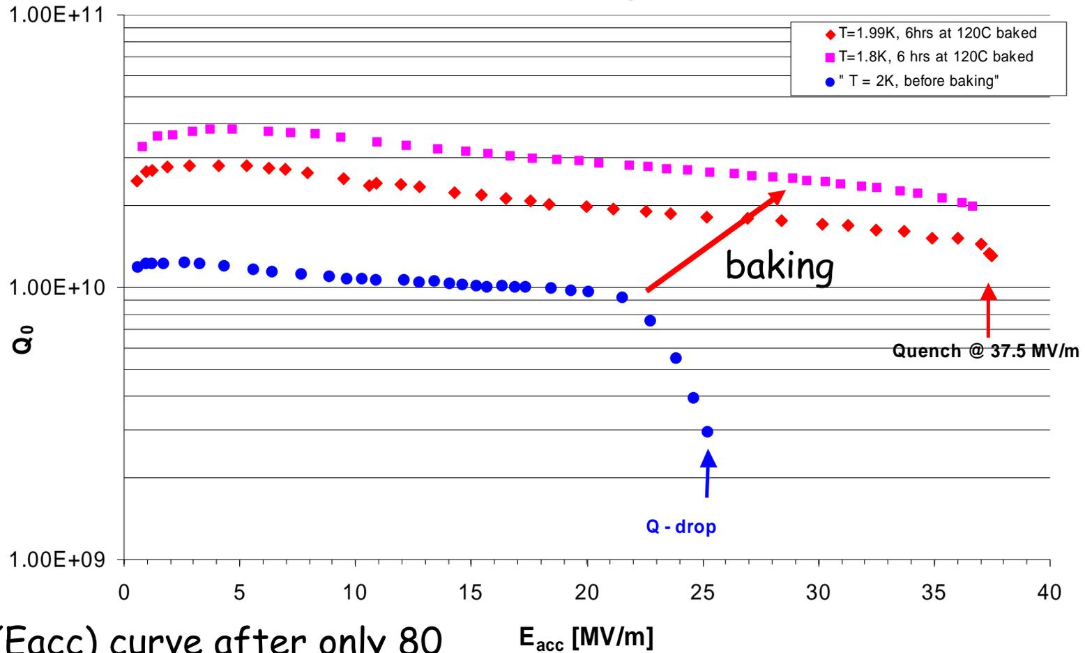
Q( $E_{acc}$ ) curve after only 80  $\mu\text{m}$  BCP and in situ baking 120°C for 12 hrs.
