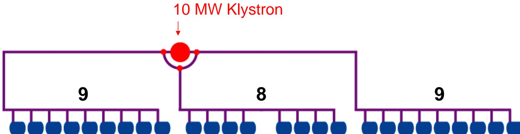
$$33.5 \text{ MV/m} * 9.5 \text{ mA} * 1.038 \text{ m} = 330.3 \text{ kW} \text{ (Cavity Input Power)}$$
